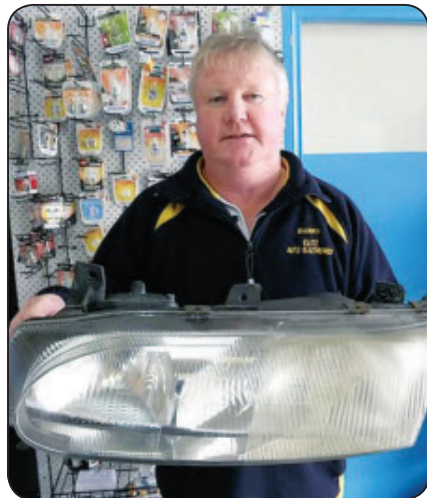
Barry with a headlight lens where the right hand side is the untreated lens and the left hand side after the cleaning treatment has been undertaken.
